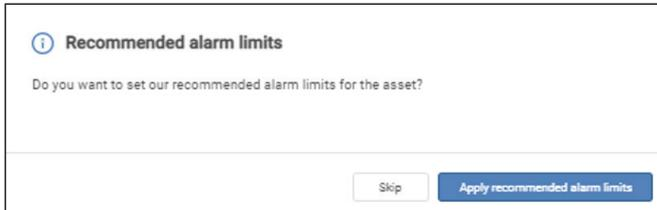
This box provides users the option of having the software set the alarm limits automatically based on a specific asset's information. The ability to have auto-generated information is a timesaver. It sets thresholds for the captured vibration measurements, including overall velocity and trends (velocity bands and acceleration bands).
