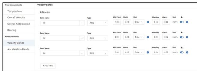
Think about a car's flexibility with an automatic transmission that you can also drive with a manual shift. The auto-generated thresholds based on machine details are highly beneficial for those with a beginner to intermediate experience level. And users with more experience can add additional customized bands manually.
